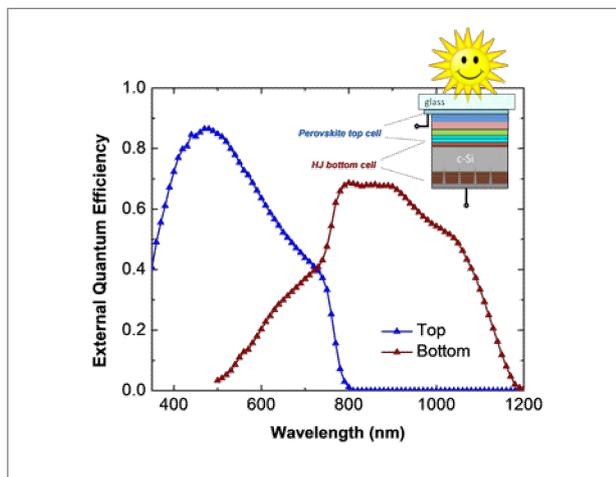
Fig. 1 Quantum efficiency of a tandem cell
