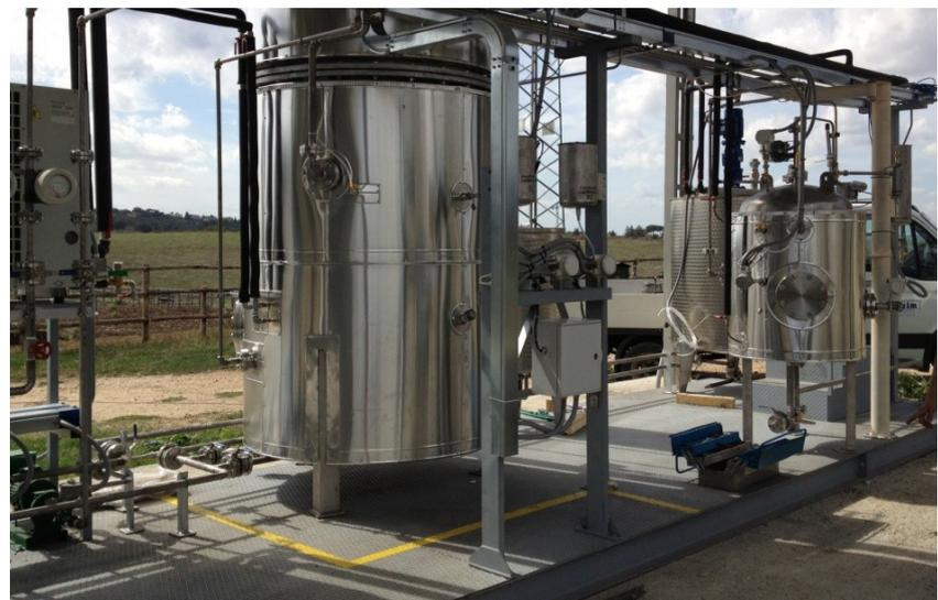
Fig. 3 Two-stage anaerobic digestion pilot plant at CREA Research Centre in Monterotondo
