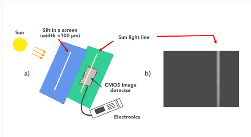
Fig. 3 Schematic of the Sun detector of the ENEA compass (a): the bright line projected on the CMOS detector is a 1D image of the Sun (b)
