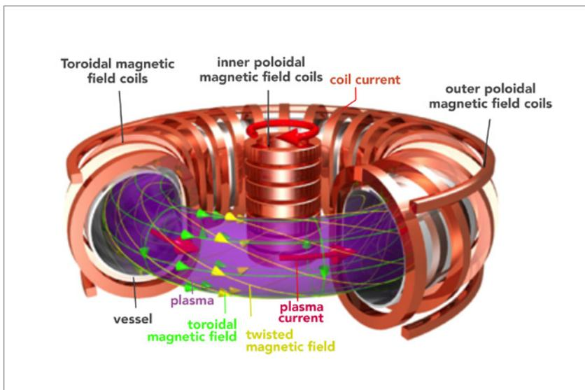
Fig. 1 Schematic view of magnetic confinement in a Tokamak
