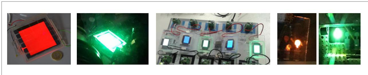
Fig. 3 Other ENEA NANO OLEDs of various shapes, dimensions and colours
