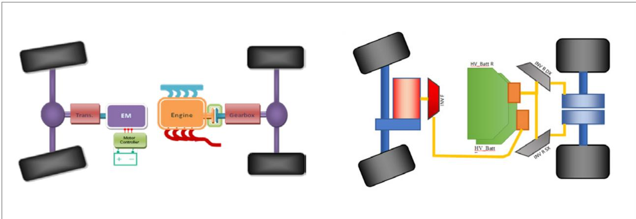
Fig. 1 and 2 Hizev hybrid layout (left) and Hizev electric layout (right)
