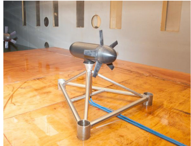
Fig. 2 Left: 1.5 m diameter model turbine during wave/current interaction tests in the wave tank (Courtesy Schottel Hydro GmbH); Right: Two 0.4 m model turbines during simulated turbine operation in array in the Circulating Water Channel (Courtesy SABELLA SAS)
