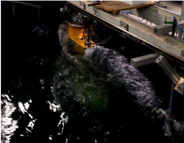
Fig. 2 Left: 1.5 m diameter model turbine during wave/current interaction tests in the wave tank (Courtesy Schottel Hydro GmbH); Right: Two 0.4 m model turbines during simulated turbine operation in array in the Circulating Water Channel (Courtesy SABELLA SAS)
