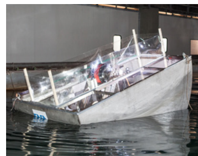
Fig. 6 PEWEC 1:12 prototype during test operations in the towing tank in Rome
