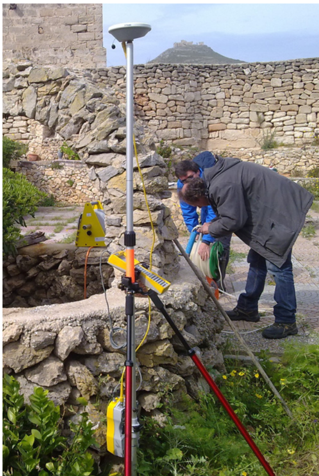
FIGURE 5 Measuring the DGPS position and elevation
