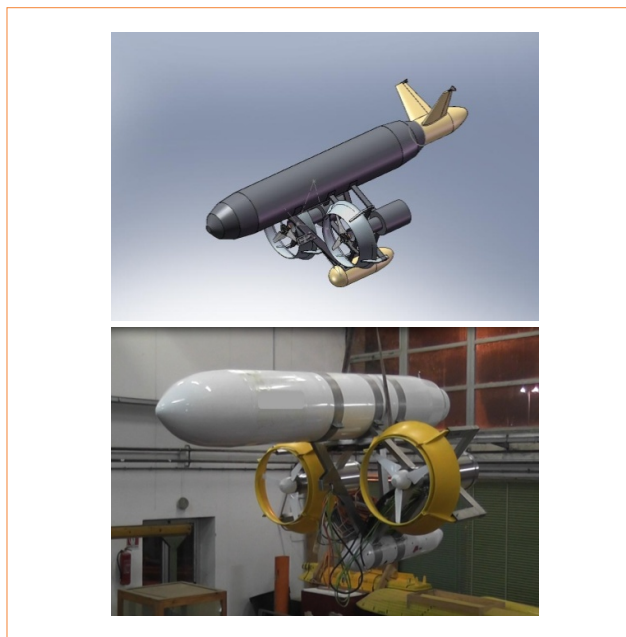
FIGURE 3 GEM prototype for towing tank tests. Scale 1:8
