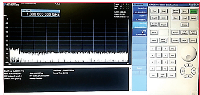
FIGURE 15 Image of the RF spectrometer screen before the excess power event (sample L122(120-160))
