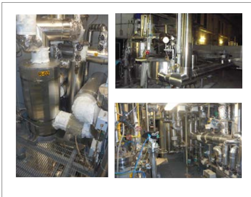
Fig.5 The molten salt heated pilot membrane reformer built in ENEA Casaccia research center (project CoMETHy)
