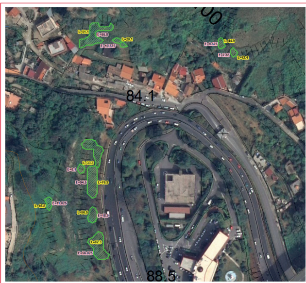
FIGURE 5 Very high susceptibility areas (green) with the propagation distances expressed in meters (yellow) and the maximum kinetic energy expressed in thousands of kilojoules (pink)
