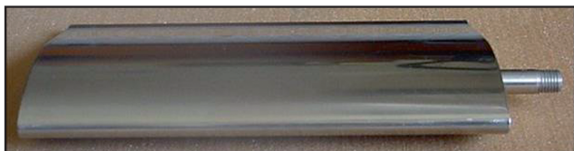
FIGURA 6 Real-scale propeller profile coated with nanocomposite Ni deposit containing SiC NPs prepared at ENEA by laser pyrolysis Source: results of PROCOMP-RINNOVA Project at the Univ. of Trento, Italy [13]
