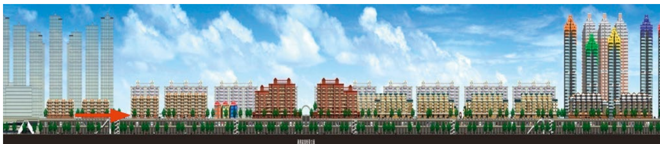
FIGURE 15 Group of 48 isolated buildings with storey isolation supported by a unique r.c. platform
