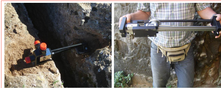
FIGURE 3 3D joint meter installed on the giant joint of the plateaux of the west side of Cala Rossa (left) and the removable deformer during the measurement survey
