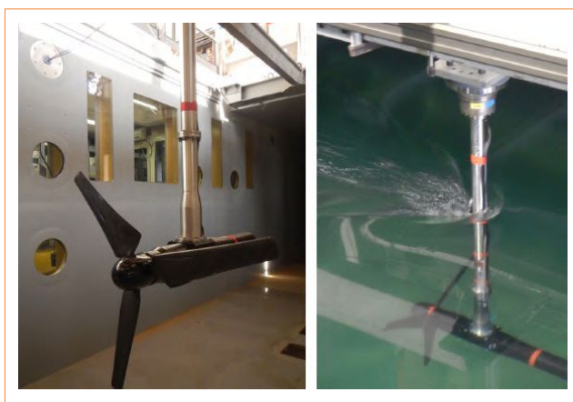
FIGURE 6 The horizontal-axis, 3-bladed rotor designed at IFREMER (France) used in the Round-Robin tests. Pictures show trials at CNR-INSEAN water flume (left) and towing tank (right)
