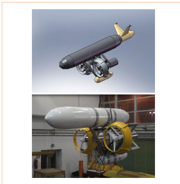
FIGURE 3 GEM prototype for towing tank tests. Scale 1:8
