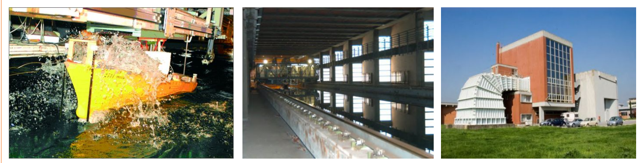
FIGURE 1 CNR-INSEAN facilities for hydrodynamic testing of marine renewable energy systems. From left to right: wave tank, calm-water tank and circulating water channel
