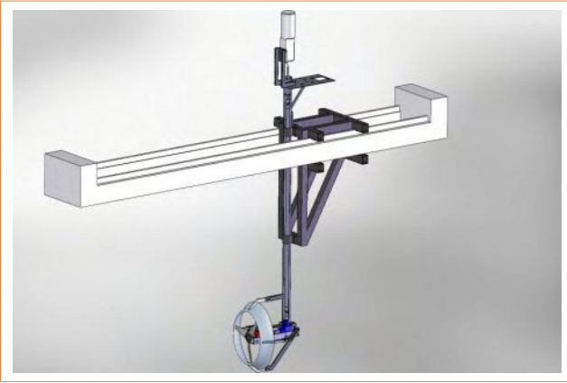
FIGURE 9 CAD view of the testing structure for an isolated turbine
