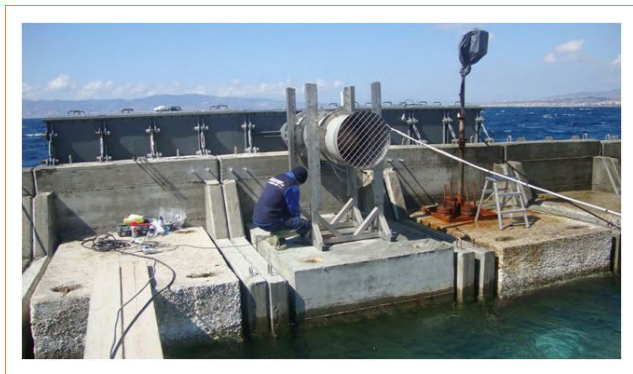
FIGURE 2 Wells turbine installed at the REWEC3 breakwater at NOEL laboratory. The turbine has been designed within the POSEIDONE project by the team of the University of Rome La Sapienza and manufactured by Faggiolati Pumps SpA. Experimental activities are managed by Mediterranea University and Wavenergy.it
