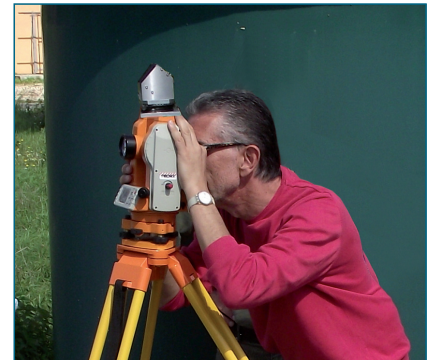
FIGURE 3 The ENEA compass mounted on a theodolite during the measurements performed at Doganella's aquifers in Rocca Priora (Rome), under a collaboration agreement with ACEA
