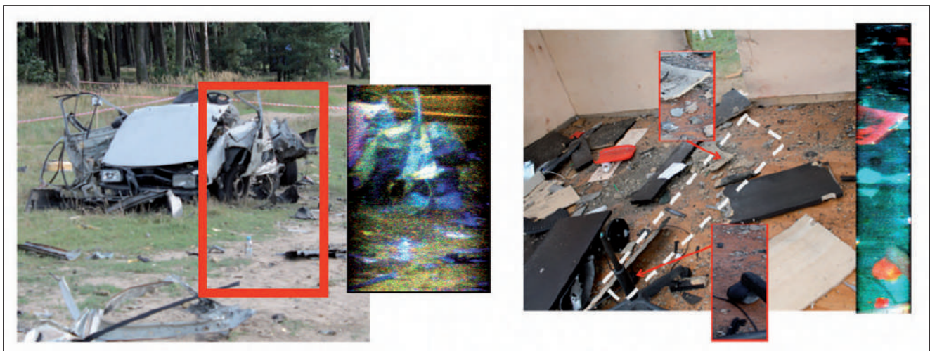
FIGURE 9 Fluorescence images of areas of the outdoor (left) and indoor (right) scenarios reconstructed by the RGB method
