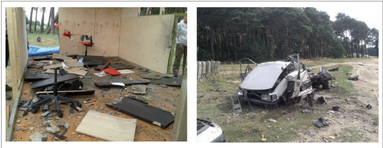
FIGURE 8 Post-blast outdoor and indoor scenarios in Wroclaw's test
