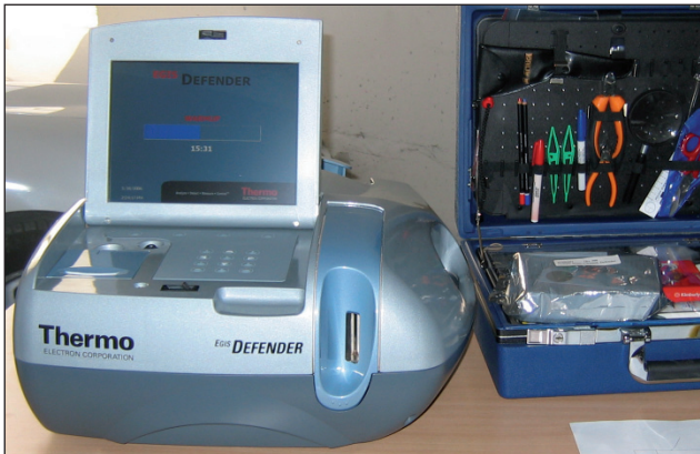
FIGURE 1 Portable explosive detector used in criminal investigations in Italy. Courtesy of G.G. Vadalà
