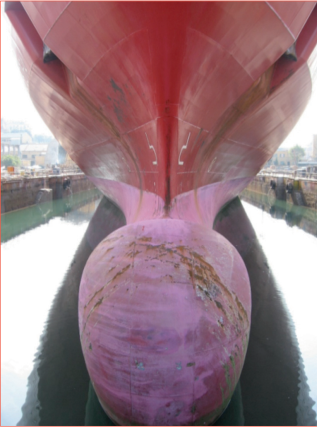
FIGURE 3 The hull of a ship protected with biocide-based antifouling coatings (Photo of M. Faimali)
