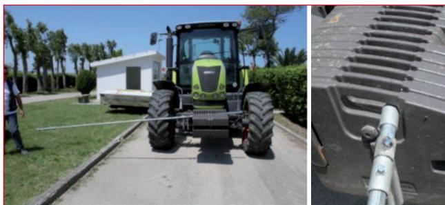
**FIGURE 3** Fledging bar installed on a tractor of the Di Vaira farm. Right: detail of the bar hook
