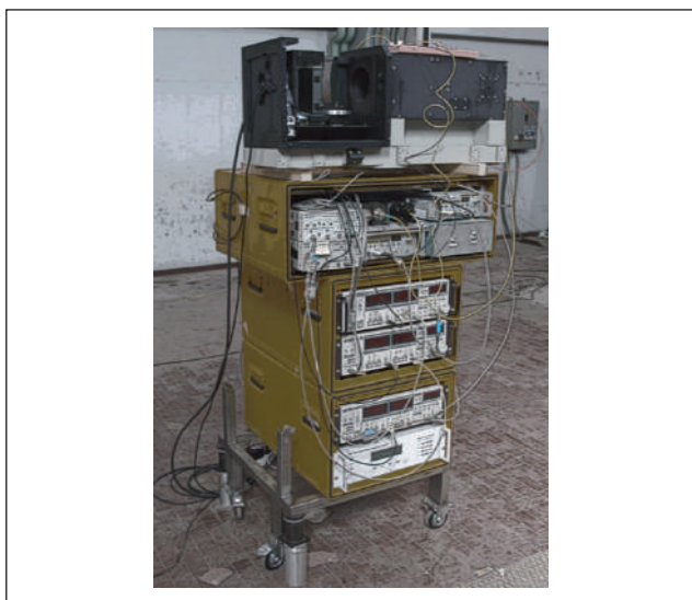
FIGURE 1 RGB-ITR scan system in tower configuration. Lasers and electronic units are allocated in the yellow boxes, while the optical head is above Source: ENEA
