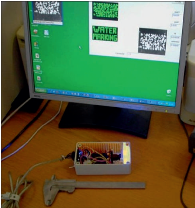
FIGURE 4 Prototype of a portable reading device able to detect the invisible images placed on a desk. On the PC screen there is the coded data matrix (a 2D binary array) transmitted by the ENEA device as read on the irradiated film, and below the corresponding sign “WATERMARKING” as decoded by a specific software
