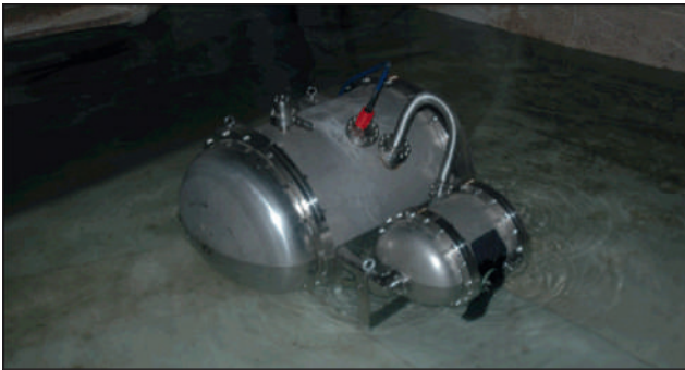
FIGURE 4 Photo of the RE-VUE system used for underwater 3D imaging. The small cylinder contains the laser source, the scanning system and the receiving stage (lens and fast photomultiplier). The big cylinder, instead, hosts the electronic modules (e.g., lock-in amplifier) Source: ENEA
