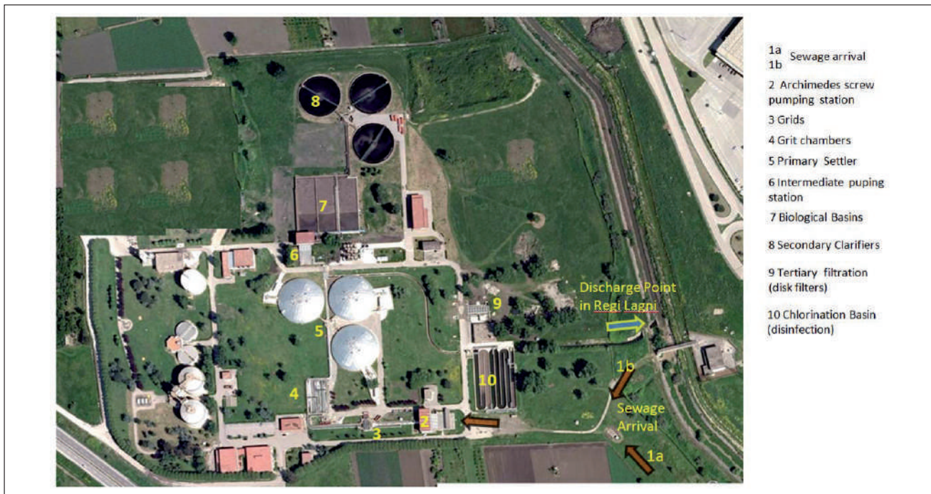
FIGURE 2 Aerial view of the plant with the legend of the main wastewater treatment sections (Water Line)
