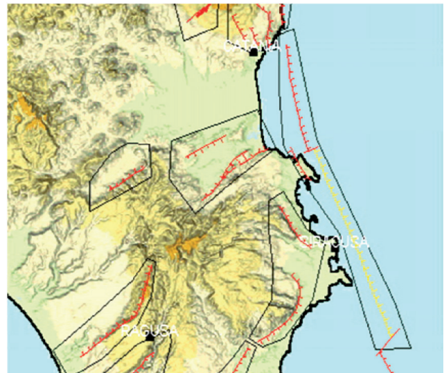
FIGURE 3 Seismogenic tectonic structures of interest for the definition of the VGM at Augusta-Priolo Gargallo Source: APAT, 2004
