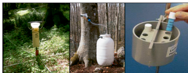
FIGURE 5 Sampling instruments: collector for precipitation quantity- stem flow - ozone Source: CNR
