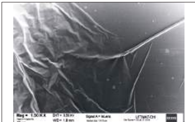
FIGURE 6 Multilayered graphene film showing corrugated morphology Source: ENEA
