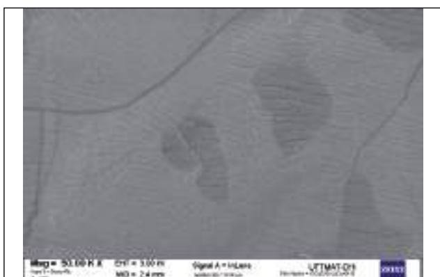
FIGURE 8 SEM image of Cu substrate after graphene growth with ethanol precursor Source: ENEA
