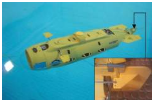
FIGURA 1 Balance positioning to dive the submarine and lock the rudder system Source: ENEA
