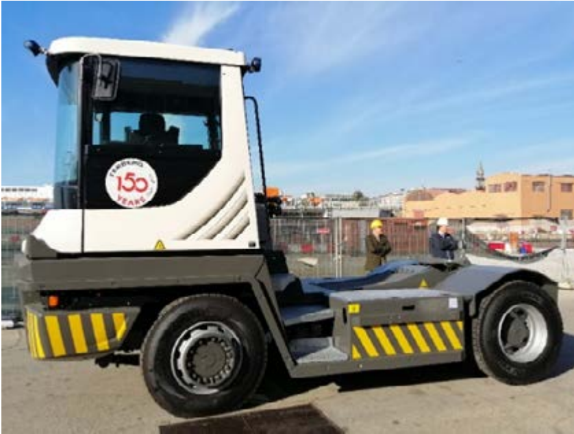
Fig.3 Yard Truck for port operation [3].
